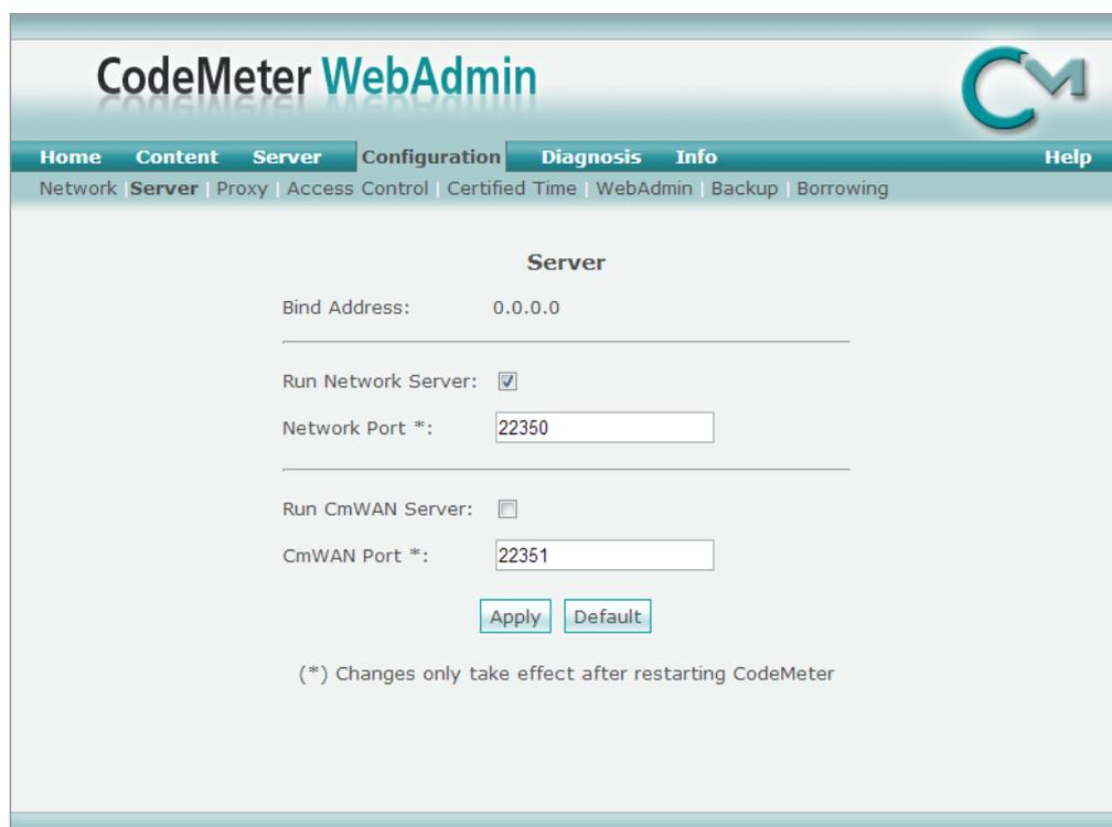
**Figure 3.8.** Codemeter Server tab within Codemeter Configuration, showing network license server configuration.
